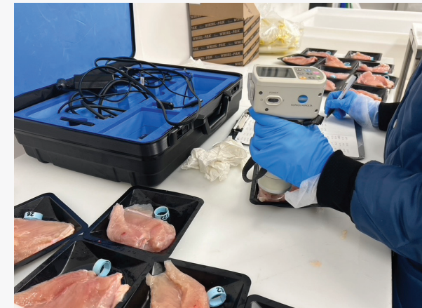
Researcher using a chroma meter to objectively measure the color of chicken breasts to assess quality.
