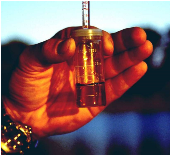
Figure 3. Test your water for alkalinity so that lime can be applied in the winter.
