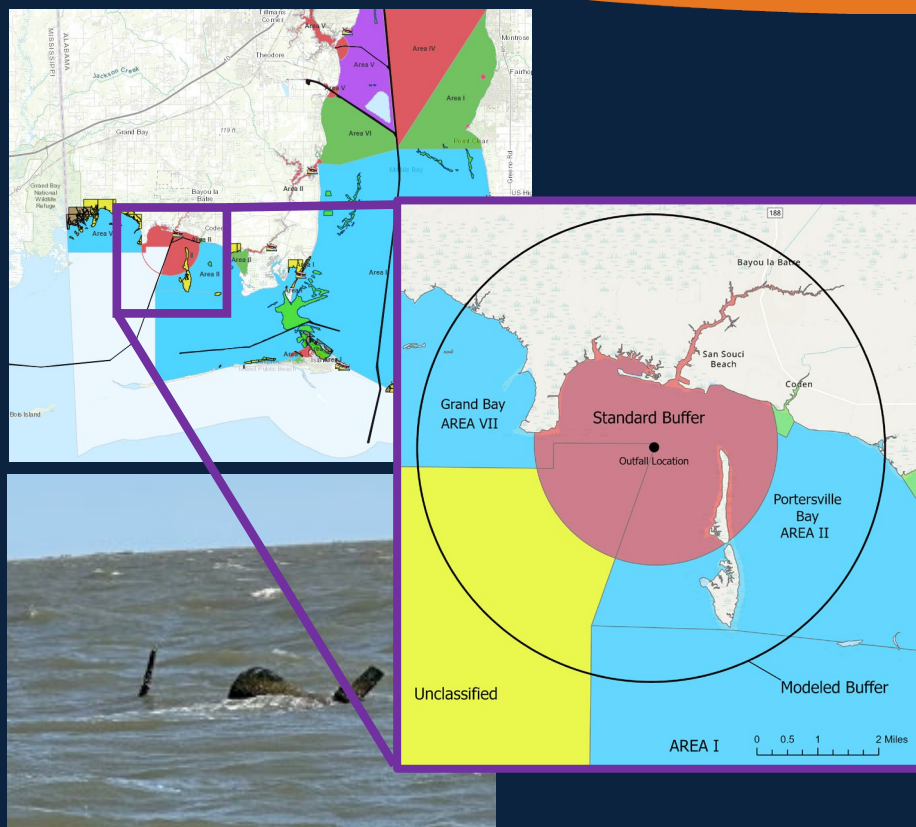
Map showing approved oyster growing areas (blue), restricted growing areas (green), unclassified areas (yellow), and prohibited areas (red). The standard buffer around the Bayou. La Batre wastewater treatment outfall (red circle around black dot) helps ensure that oysters harvested from nearby Portersville and Grand Bay are safe for human consumption. New models that incorporate the outfall at the surface suggested that the buffer be extended out to 3.8 miles from the outfall (black ring). Photo: The Bayou La Batre Wastewater treatment outfall could be seen at the surface and posed a hazard to navigation until it was reattached to the seafloor on May 19 th . (Photo Credit ADPH)
