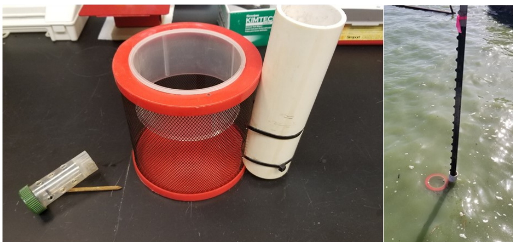
Figure 1. Basic snail trap construction (left) showing bait holder (far left). If trap was baited, a small carrot was placed inside the bait holder, which sat inside the trap itself. Traps were deployed along the pond margin, just below the water surface and secured in place using a T-post (right).
