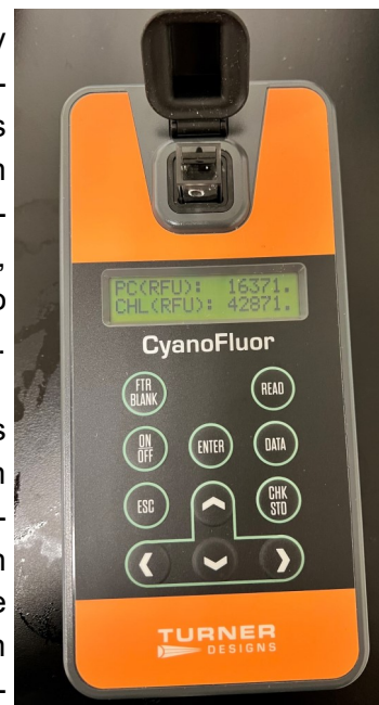
Fig. 3 The Turner Tool is used to measure the extent of the blue-green algae problem.
