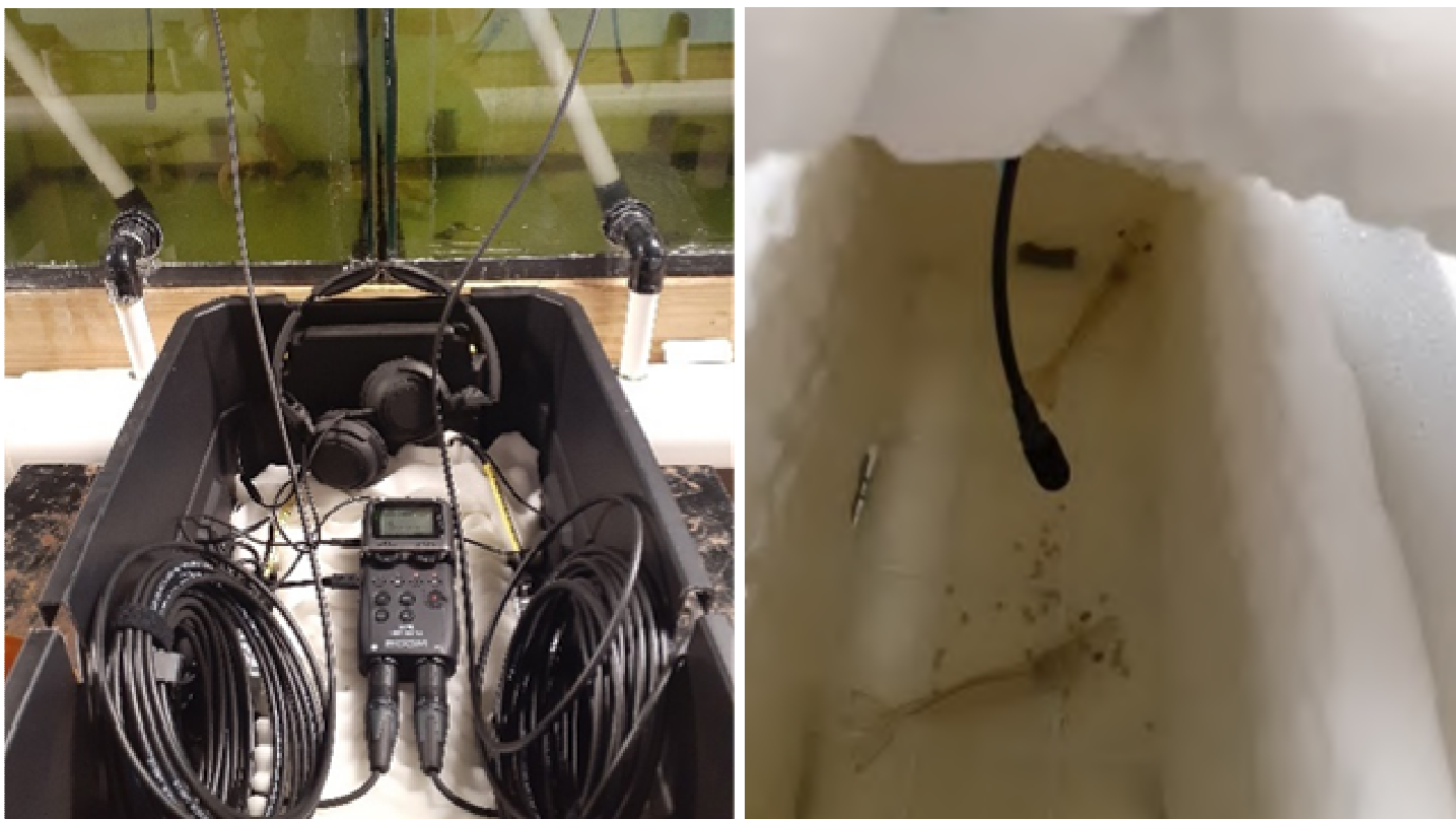
Fig. 2. Hydrophones and digital recorders used to monitor feeding sounds in glass tanks (right) and acoustic chambers (left).
